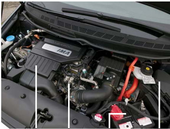
Engine Motor 12-Volt Battery Underhood Fuse Box
